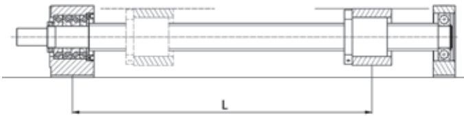
Figure 2.15 Bearing arrangement fixed - supported
