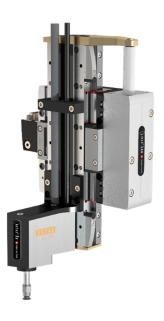
Mounting to an LINAX® Lxu ground plate Example: 1 x LINAX® Lxu160F60 1 x ROTAX® Rxvp 28-6T0.04 1 x Angle bracket for LINAX® Lxu incl. 4x torx M4 x 8 2 x Dowel bushings Ø7mm 2 x Centering pins Ø4 x 6mm
