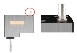
The ROTAX<sup>®</sup> Rxvp is supplied with a Ø4mm (0.16") connection plug as standard. Recommended hose inner diameter 3mm (0.12").
