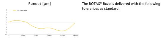
Runout radial 15mm (0.59") shaft10μrRunout radial 30mm (1.18") shaft10μr
